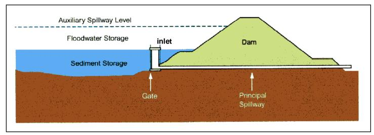
This cross section of a dam shows the concrete inlet in front of the dam connected to the principal spillway pipe (extending through the dam). When water reaches the opening at the top of the inlet it spills over and goes through the pipe controlling the level of water in the lake. Some inlets also have openings in the side of the tower.
