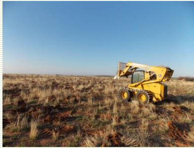
District clearing brush on producers pasture with the Marshall skid steer attachment.
