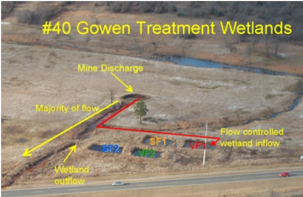
Figure 2.2. Aerial photograph of the #40 Gowen Treatment Wetlands Demonstration Project. Note the proximity to Highway 270 and production agricultural lands..
