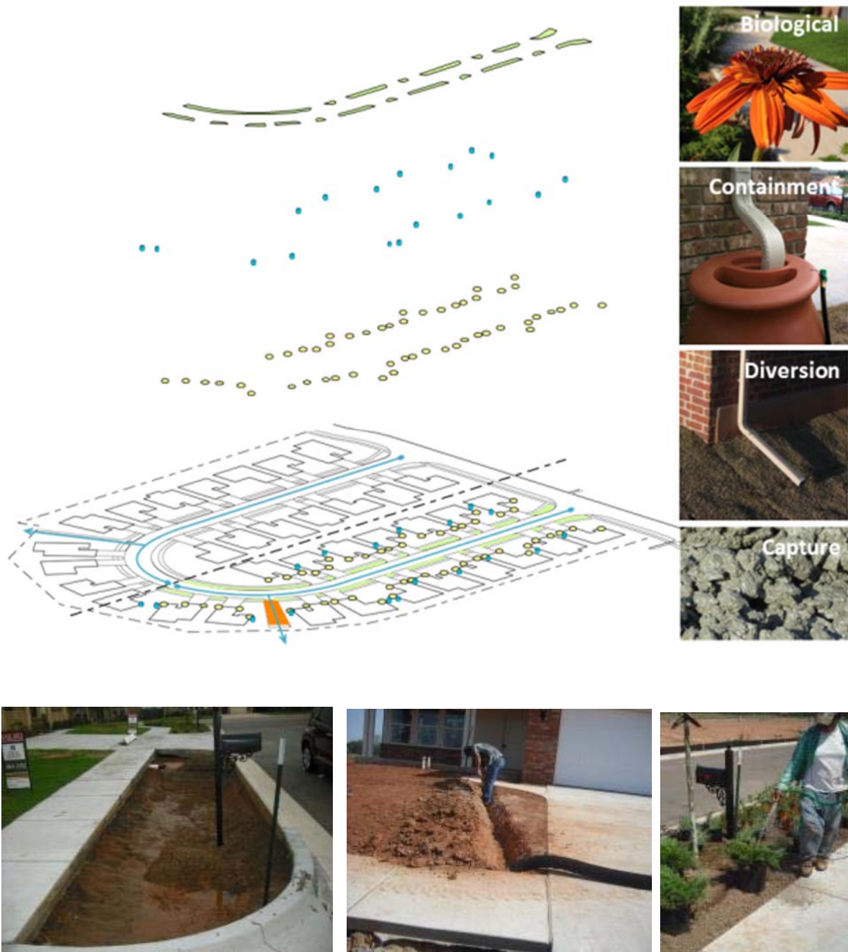
Figure 11: Shows the four BMPs per lot: Biological (rain garden), Containment (rain barrel), Diversion (downspouts), and Capture (a small section of porous pavement). Below (left) is a lot with rain garden in mid construction, a downspout diversion (middle), and plant installation (right).
