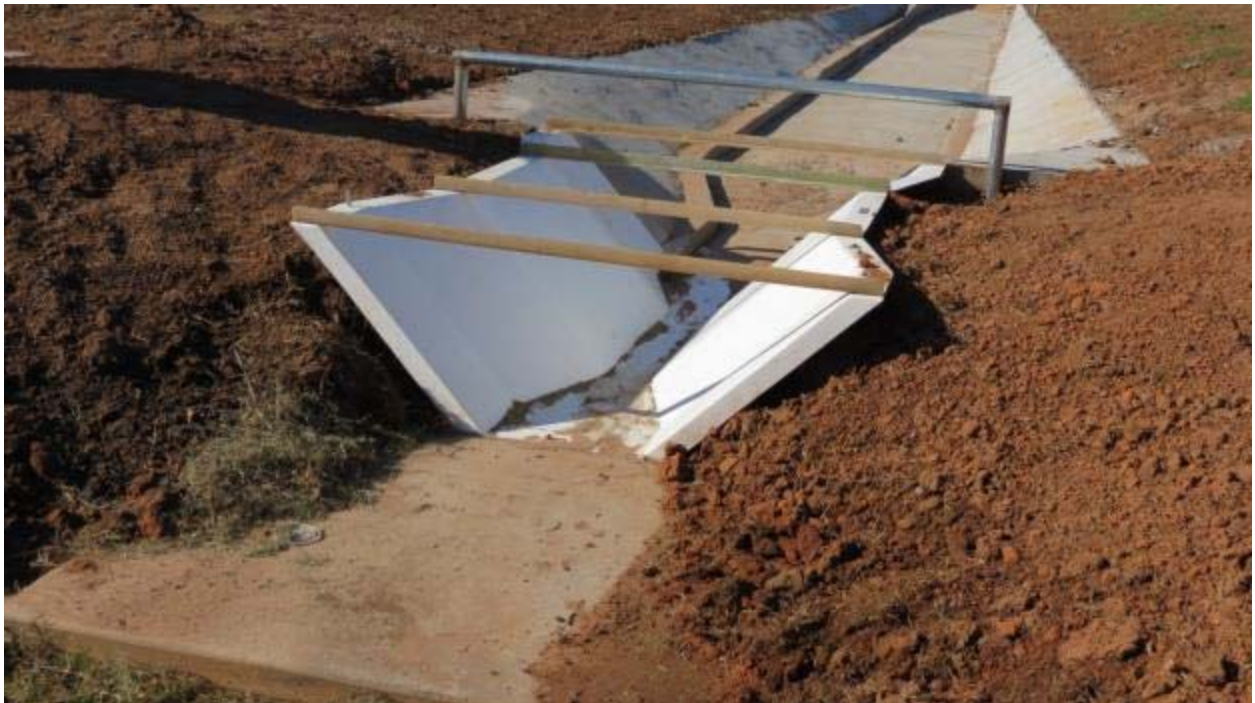
Figure 17: Photo of Plasti-fab test flumes were installed at the end of the concrete stormwater flumes and equipment closets were set adjacently on the top of bank west flume (Top) and east (Bottom).
