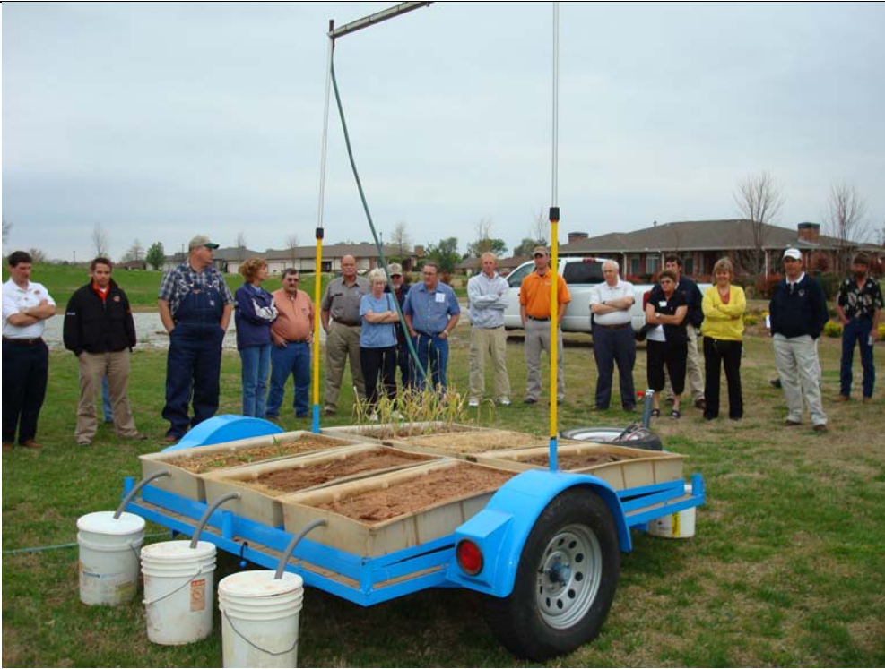
Figure 4. A rainfall simulator was used to demonstrate nutrient and soil losses from different management strategies. The amount of runoff and nutrients and sediments in the runoff varied with management, such as ground cover and amount of fertilizers applied.
