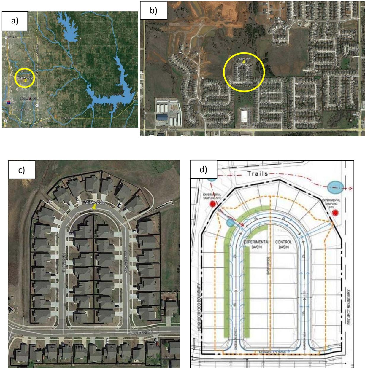
Figure 2. a) Study site location with respect to City of Norman and Lake Thunderbird, b) Trailwoods neighborhood, c) Trailwoods study site (aerial Imagery from Google Earth 2015) and d) diagram showing TE control watershed (“Control Basin”) and TW treatment watershed (“Experimental Basin”), from Coffman (2014).
