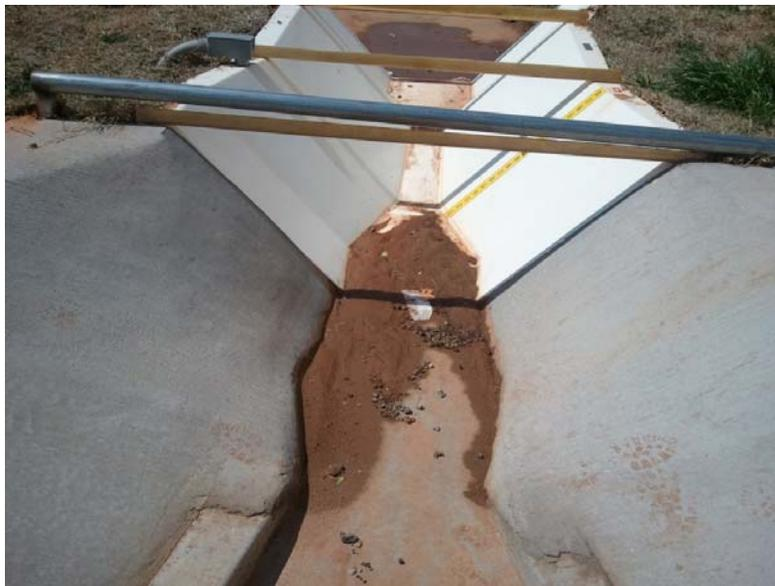
Figure 3. Installed trapezoidal test flume at downstream end of concrete stormwater flume showing downstream concrete pad. Note sediment deposition in flume from newly finished lots.
