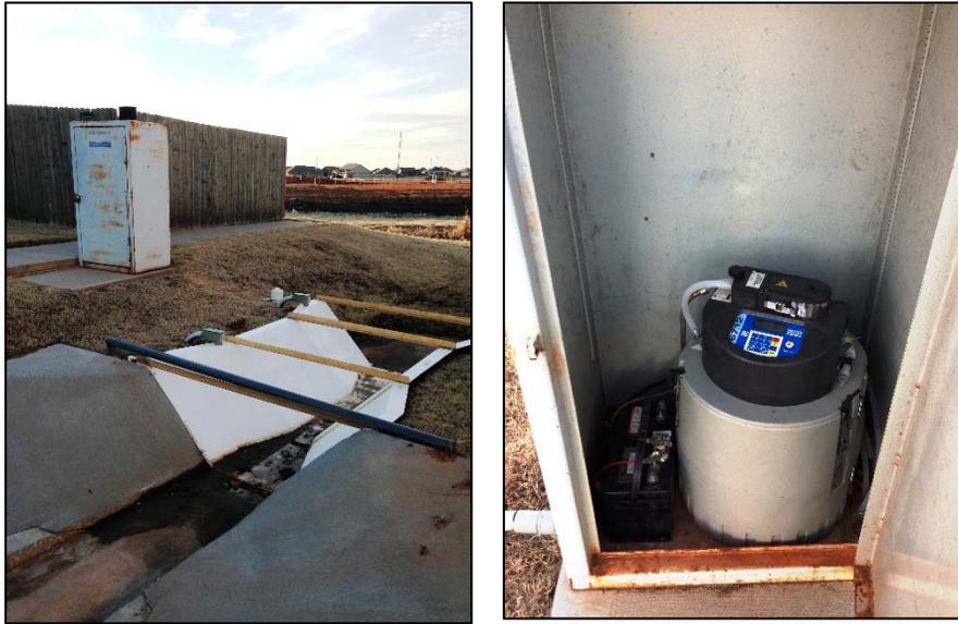
Figure 4. Trapezoidal test flume and gun safe (note buried connections between the two) and autosampler inside gun safe.
