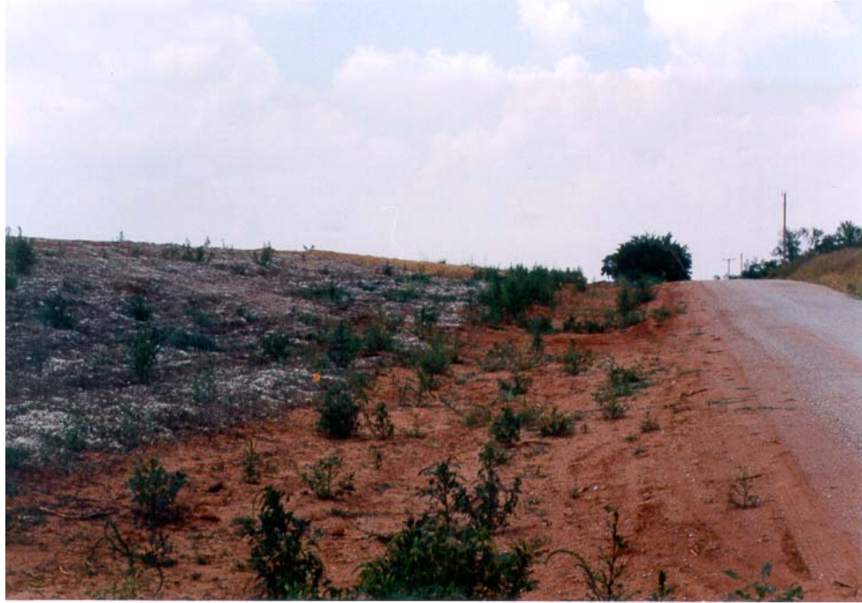
Figure 3.3 Cotton Burr Mulch at Site 1 with Limited Vegetation.
