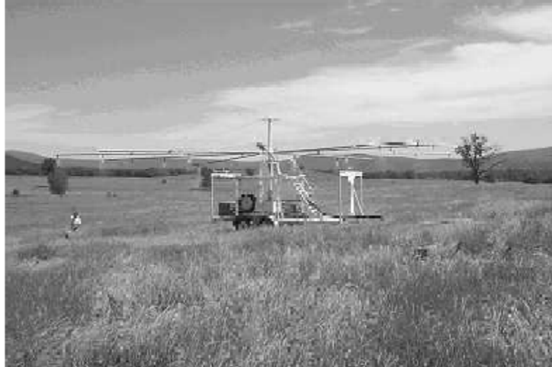
Figure 2. Oklahoma State University rainfall simulator.
