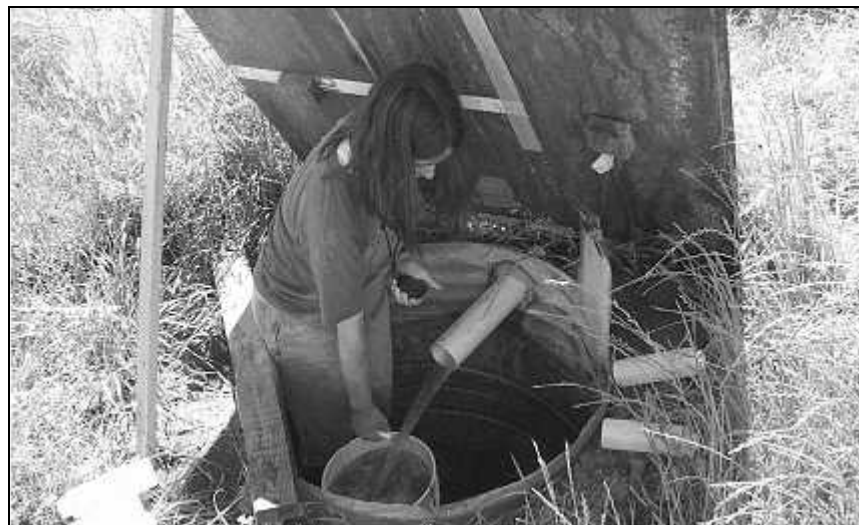
Figure 5. Rainfall simulator collection pit
