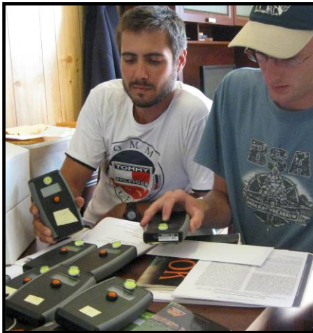
Figure 1. Optical pocket sensors with NDVI display readings on the top, and active sensor reading on the bottom.
