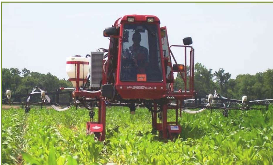
Figure 7. On-the-go variable N fertilizer sprayer developed at Oklahoma State University capable of applying prescribed fertilizer N rates to each individual corn plant.
