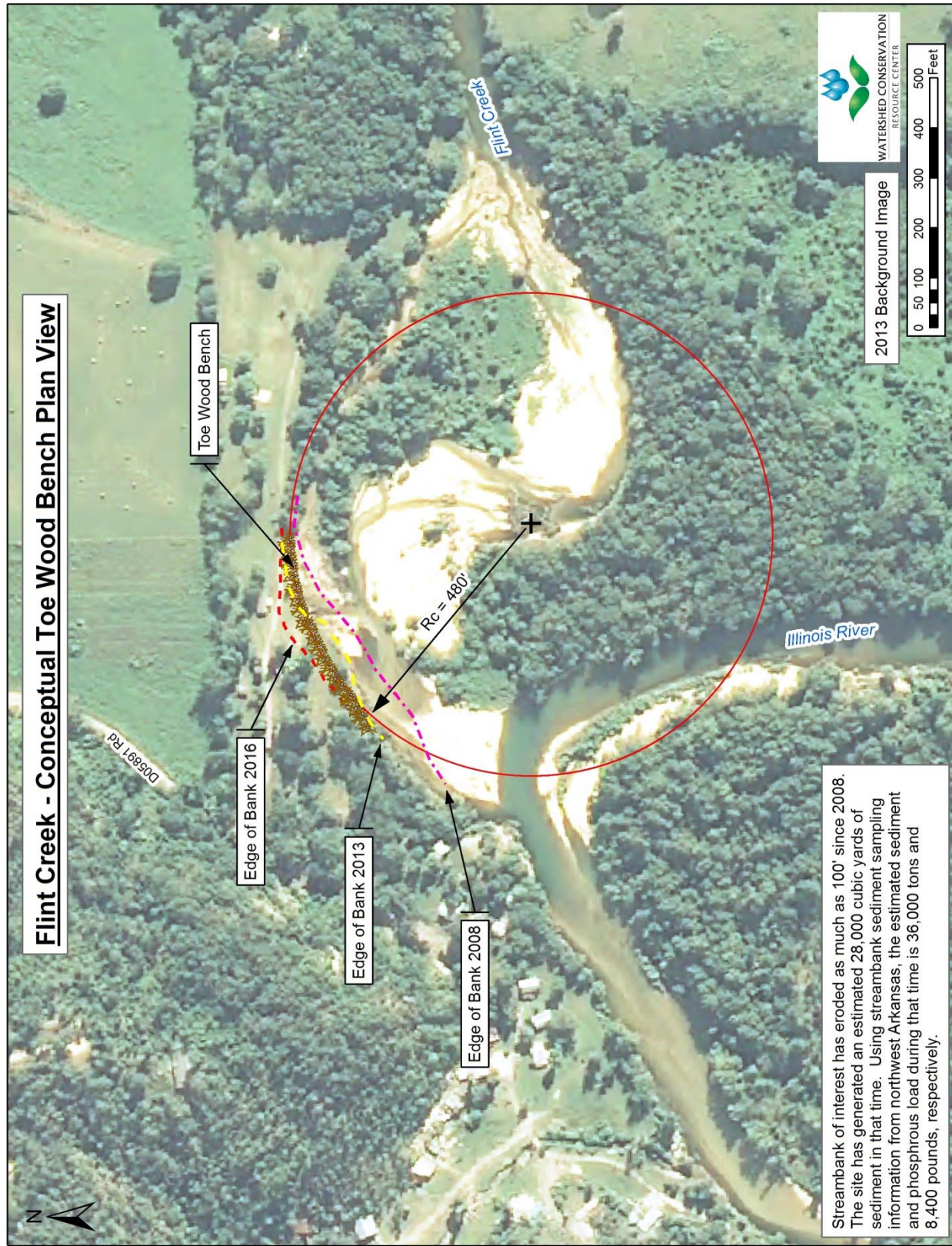
Figure 7 Conceptual toe wood bench layout for bank stabilization on Flint Creek near Dripping Springs, OK
